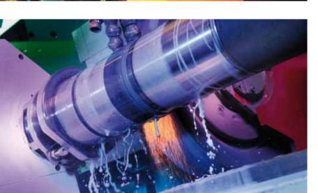
Unique combination: induction hardening and machining
